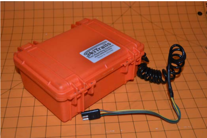
Satellite tracking unit in rugged case, for use on snowmobile grooming equipment.
