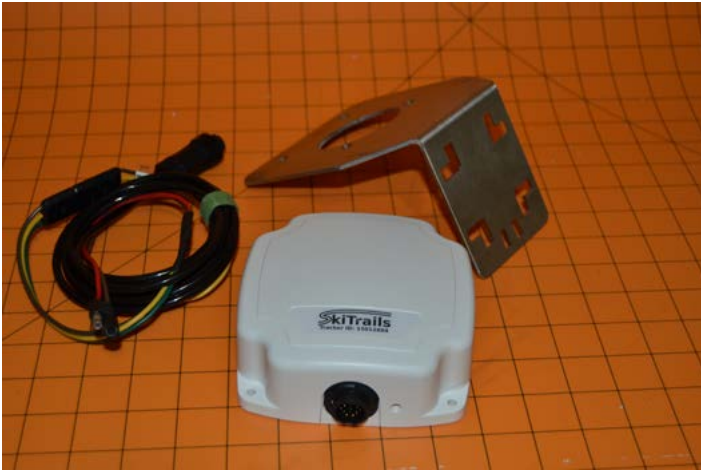
Satellite tracking unit, with pole/bar mounting bracket for use on large machines (Pisten Bully, Prinoth, etc)
