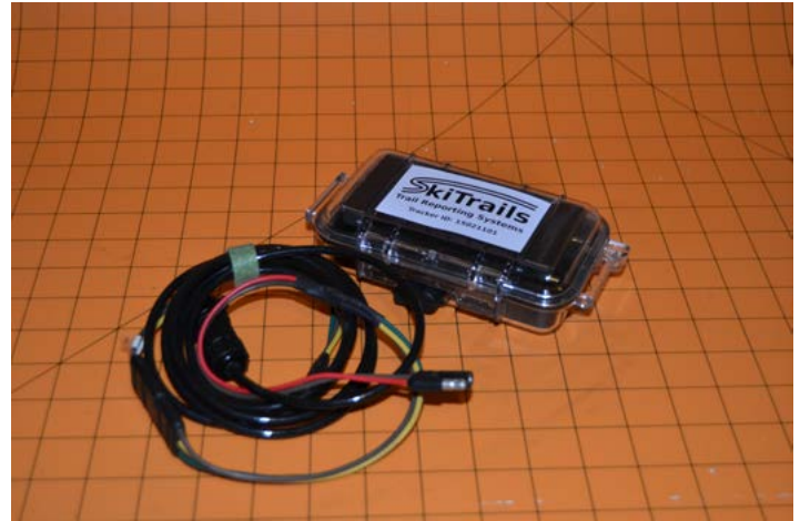
Cellular tracking unit, for use on small or large grooming machines. Lower cost, requires cell/mobile coverage.
